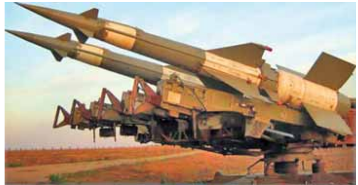
External appearance of launcher 5P73.
