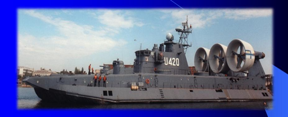
Type – gas turbine air-cushion landing ship of amphibious type.
