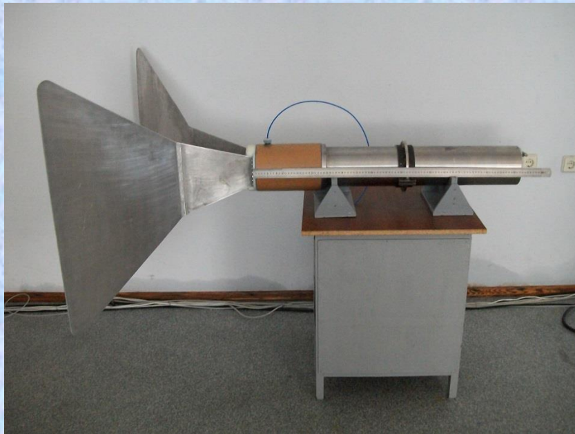
TEM-antenna made of sheet metal
