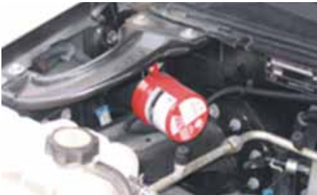
Fire-extinguishing of engine compartment
