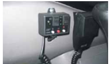
Siren and flashlights control
