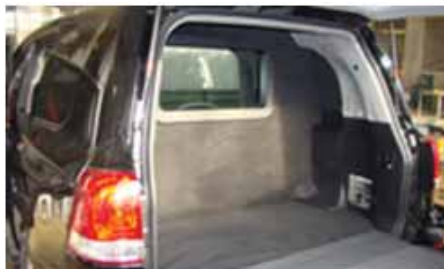
Armoured partition wall
