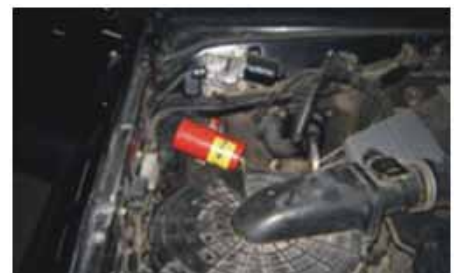
Automatic fire-extinguishing system of the engine compartment
