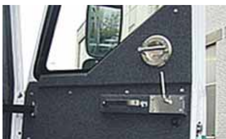
Special internal mechanical door locks (crossbars)
