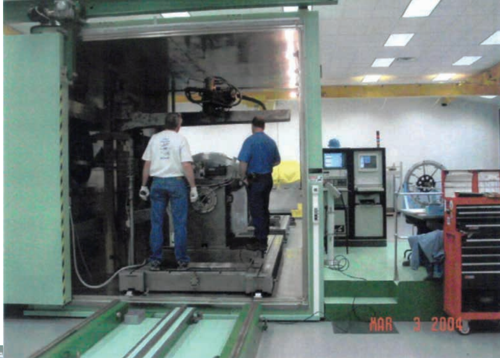
KL-115 machine and welded component of a jet engine
