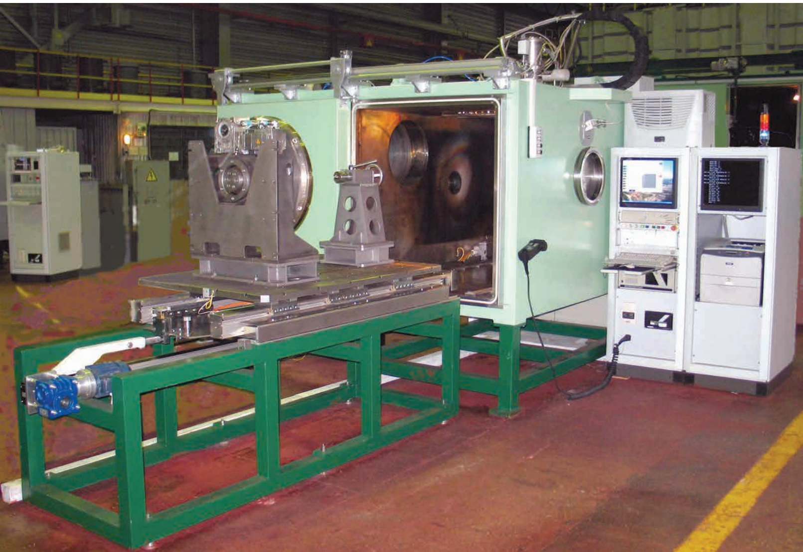
Specialized machines KL-134 with welding gun sliding on the chamber upper cover and KL-154 machine were developed for electron beam welding of titanium spherical tanks for space application.
