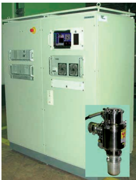
General view of both power source ELASM-120/6 and welding gun
