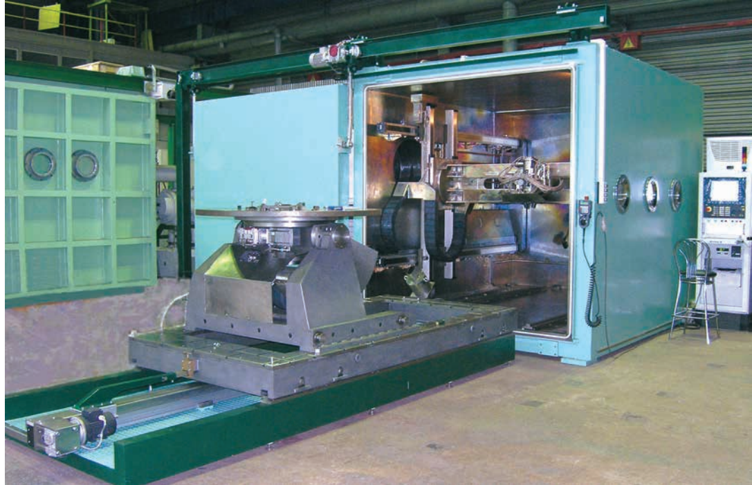
KL-132 machine was developed for EBW of jet engine components of SU-30 fighter at HAL Company plant (Koraput, India)
